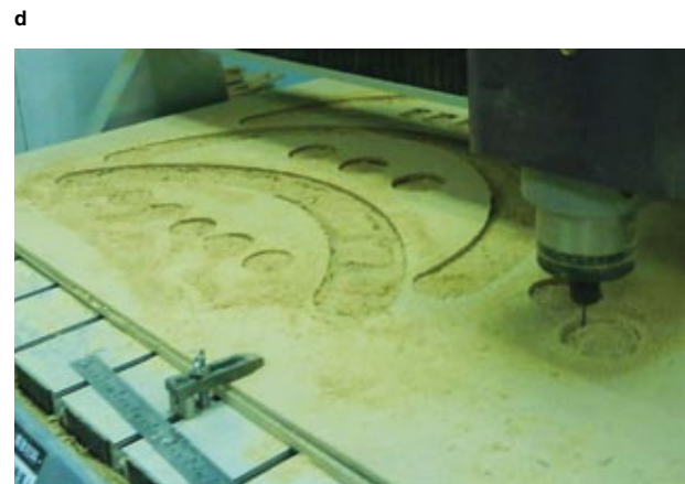
Figure 2: Four chairs in one drawings and construction by Yun-Fang Huang: (a) sections study, (b) section of onion and elevations of chair, (c) layout for fabrication, (d) the parts under milling.
