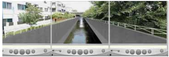
Figure 18: Panoramic view of CG animation using VR to evaluate landscape design of water way bank walls.
