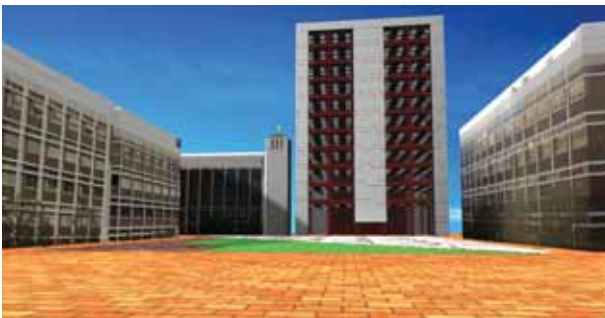
Figure 14: The new building (the tallest) is modelled in detail in 3D, while the others are simply decaled with facade photos, by Takahisa Morisaki and Azuma Seki.
