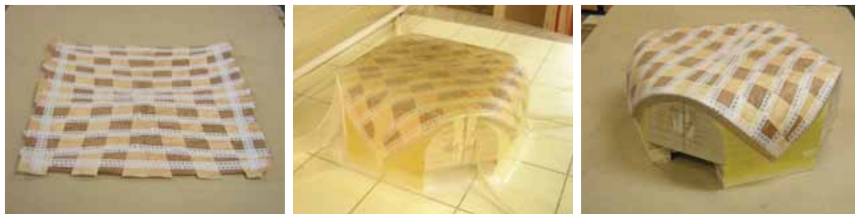
Figures 9-11: The veneer pieces are cut using templates, 'stitched' together with veneer tape and formed to a profile using the vacuum press.
