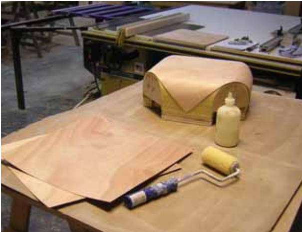
Figure 12: The layers of veneer that make up the core of the tabletop form are glued and laminated.
