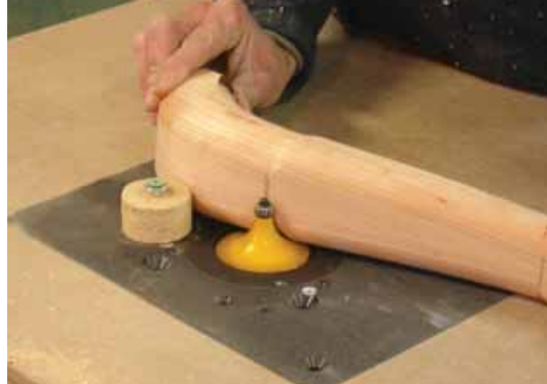
Figure 6: 'Controlled rounding' conducted using the router table.
