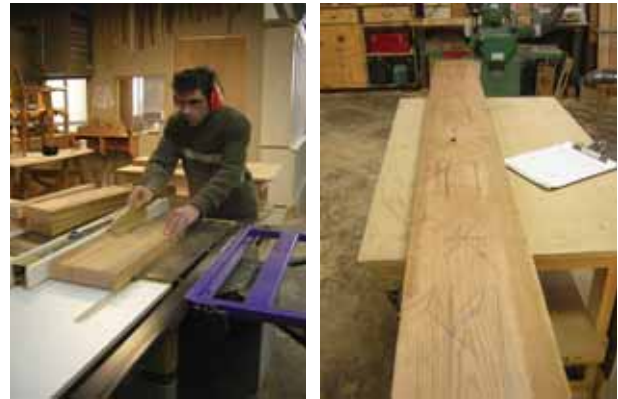
Figures 1,2: Conditioning and sizing the lumber to create 'billets'.
