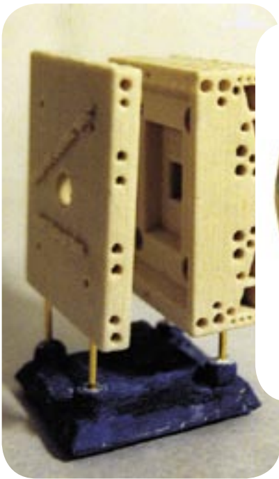
ANDREW JUNG Fine Arts Studio A typical RP mold (whose base is its casting). RP gypsum and plastic.
